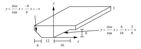
The aim is to find the volume V(y) that water occupies if it's at a height y that's less than 6 feet.
